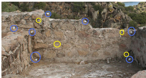
Figure 2: Image of points for georeferencing and quality control of photographs used for 3D reconstruction of the citadel. Blue circles show the small paper targets at the corners of the wall. Yellow circles show the reflective targets used as control points of the images.
